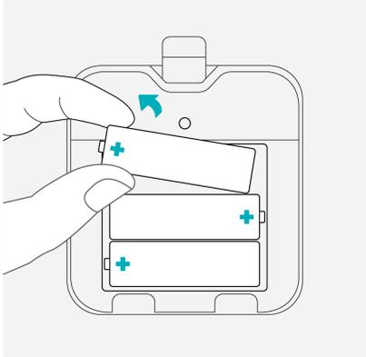
3. Insert 3 alkaline 1.5V size AA batteries as shown in the compartment.
