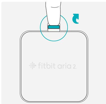
2. Remove the batteries.
